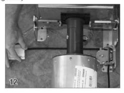
Go to the non-motor end and make sure the rope will come straight back from the rope channel of the guide to the pulley. If the ropes do not come straight back, the mechanism should be moved to balance the rope angle on both sides. Only a 1/2" variance from straight is allowed on either side.
