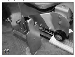
Feed the wheel assembly and cover into the guide.
