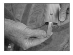
Tap the spring pin (31) into the round splice channel. Slide the center splice (30) into the center channel.
