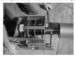
Align the mechanism on the motor side first by using a piece of rope. Extend it from the outside channel of the guide to the pulley to make sure the rope will feed directly into the pulley.
