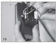
Insert the RED DIRECTIONAL WIRE into terminal B1, and tighten the screw. Note: Reverse directional wires if the cover runs opposite to the direction indicated on the switch.
