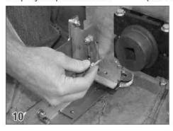
Use a 7/16" wrench to tighten the nylock nuts. Additional carriage bolts (27) and nylock nuts (29) are provided and can be used as reinforcement for the pulley brackets if needed.
