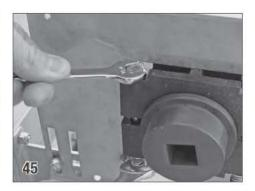
The non-motor brake should be tight enough to prevent the cover from rolling off the tube faster than it is being pulled into the guide. To adjust this brake, use two 7/16" wrenches and tightening or loosening the thru bolts in the brake block.
