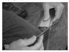
File the guide ends on both sides of the pool making sure to round all edges and remove all burrs. This step is extremely important. The cover can damaged very easily by metal burrs and this damage is not covered by the warranty.
