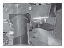
Adjust the position of the pulley brackets to raise the roll up tube to prevent the cover from rubbing on the deck.
