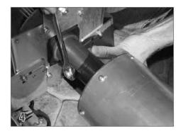
Make the same attachment by inserting a half inch bolt (28) through the hole in the split cone on the non-motor side. Secure with a nylock nut (23). Now the mechanism is assembled and ready tobe positioned near the pool.
