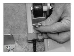
Place a bonding lug (16) on top of the guide feed. Insert a 10-32 x 1 5/8 screw (34) through the lug, guide feed, and track. Install a 10-32 nylock nut (21) and tighten with a 3/8" wrench.
