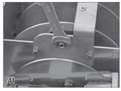
If you need to adjust the brakes, first loosen the jamb nut on the side of the rope reel mechanism.
