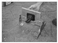
Position the motor and non motor end so the pulleys are near the pool deck.
